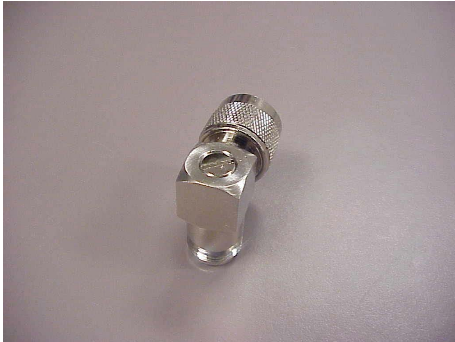
Figure 1. N-type adapters – susceptible to moisture effects
