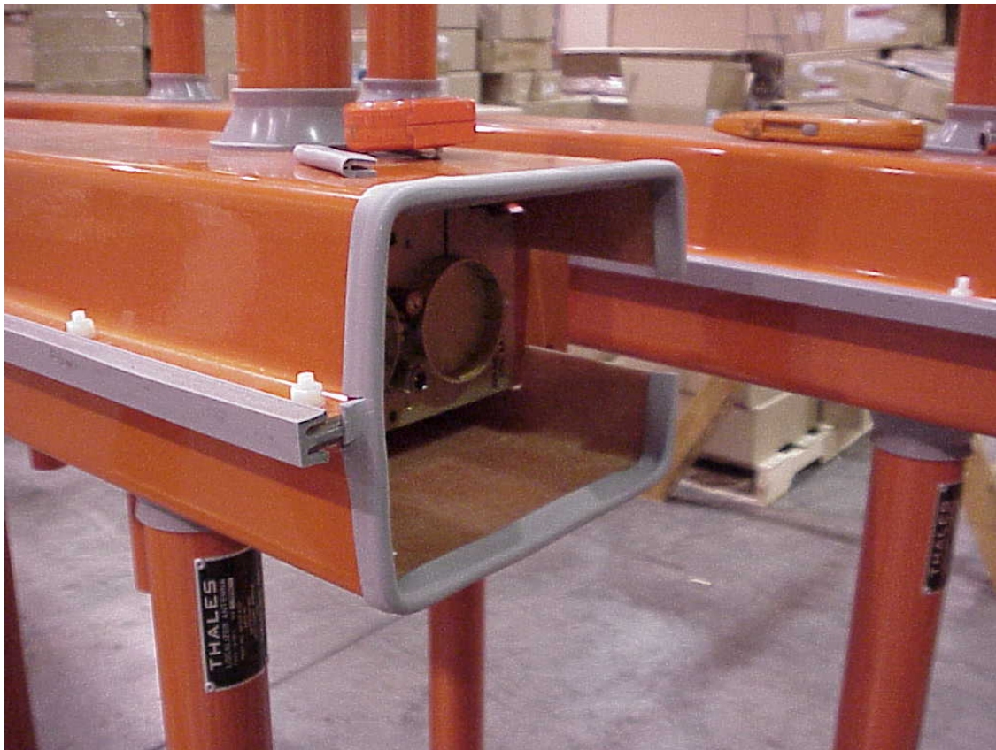
Figure 2.0. Example of Gasket Installation on Weather Shield Lip (with modifications made)
