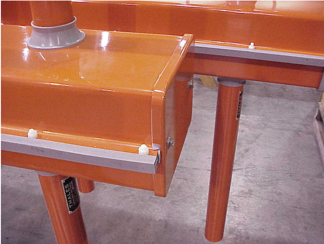
Figure 3.0. Example of Properly Installed Gasket
